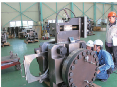
Pressure Test (API 598)
