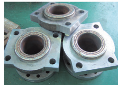
Weld Built up (ASME Sec. IX)
