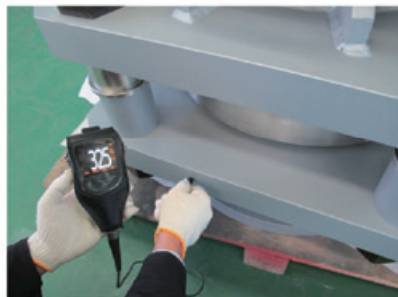
Dry Film Thickness Inspection (ISO 19840)
